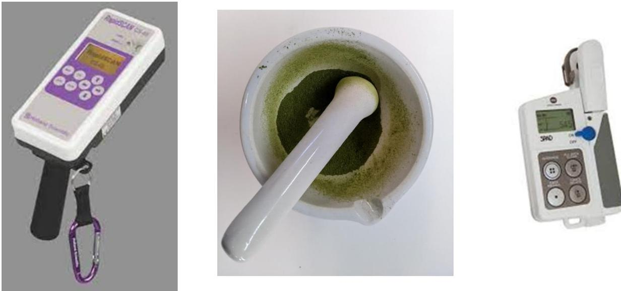
Figure 2. RapidScan CS-45 used for NDVI (left), example of a ground leaf sample (center), and the SPAD-502 leaf chlorophyll device (right).
